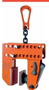
The CNMA clamp is equipped with 2 clamping jaws that are provided with special synthetic plastic. After hoisting, the clamp leaves no damage. The clamp is locked in the closed and open position.
